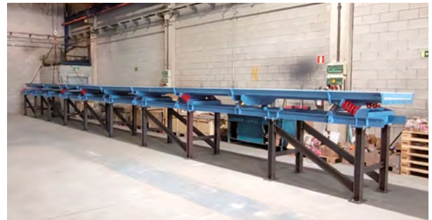
Spill sand vibrating conveyors (AMC & SBC sand collect)
