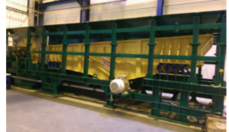
Vibrating feeders for scrap cleaning installations
