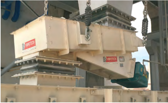
Electromagnetic discharge feeders
