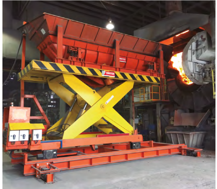
Rotary furnace charger
