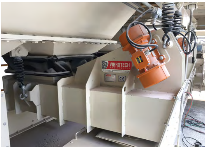
Electromechanical extractor hopper
